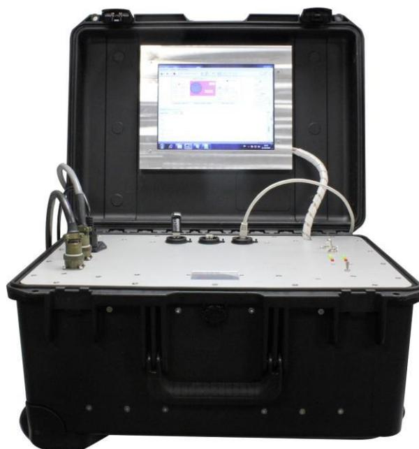
**Figure 1.-** Overview of the control suitcase of the GPC air-transportable analyser .
