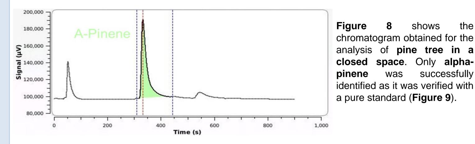
Figure 8: Chromatogram obtained for the analysis of pine tree on the portable analyzer
