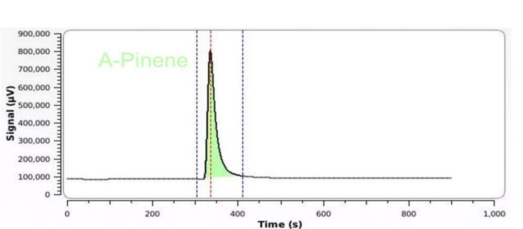
**Figure 9**: Chromatogram obtained for the analysis of pure alpha pinene
