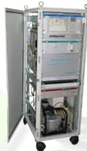
Purge & Trap cabinet
