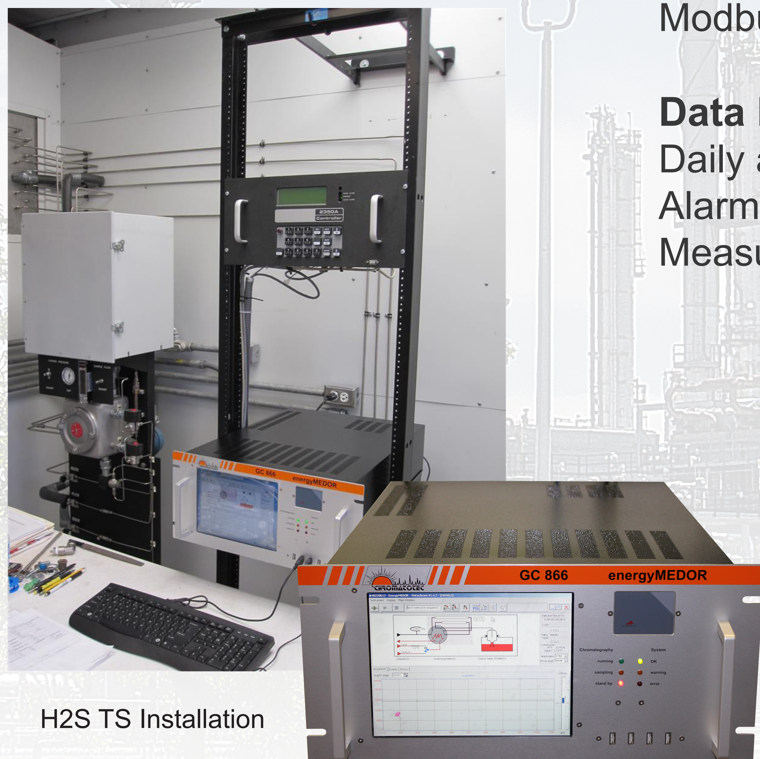
Wall mounted MEDOR analyzer GC866 ATEX Ex II 3G Ex pz IIC T4 or CSA Class 1 Div. 2 Group B, C & D
